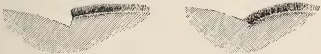
69. A common form of edge for walk or drive. 70. A better form.
